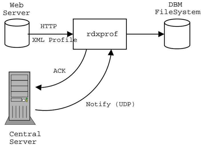
Figure 1.2: Detail of XML file transfer over UDP
